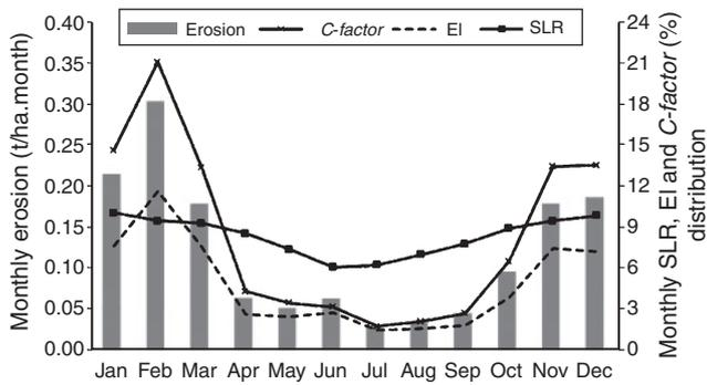
Fig. 6. Seasonal variations of *C-factor* in NSW and its relationship with hillslope erosion. EI, Percentage distribution of monthly rainfall erosivity index; SLR, monthly soil loss ratio.
