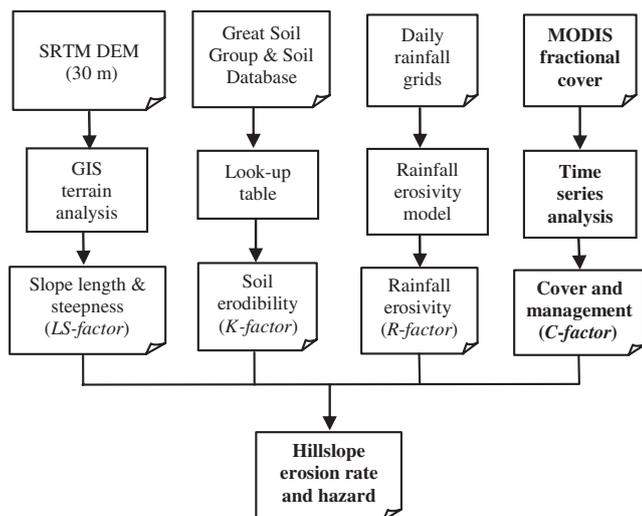
Fig. 2. Procedures for deriving RUSLE cover factor (shaded area) and hillslope erosion modelling in NSW.
